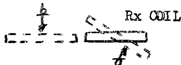
Effect of short cable or tilted coil
