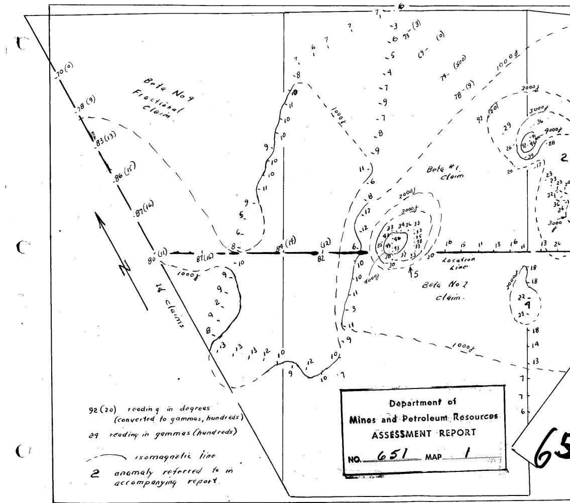
20000 ίĎ - 25 26 26 25 Beta # 3 20 Fraction 19 claims 7000 Jankana -<del>-</del> 3 200017 20001 Fig. 1 BETA GROUP showing Isomagnetic lines Scale 1"= 300' Aug 29, 65 by J.M. Black P.Eng 1/Slm
