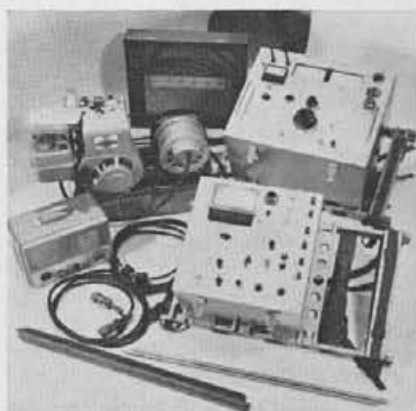
Figure 3.—(above)—The Seigel Mk V Induced Polarization Unit.
