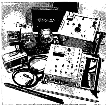
Figure 3.—(above)—The Seigel Mk V Induced Polarization Unit.
