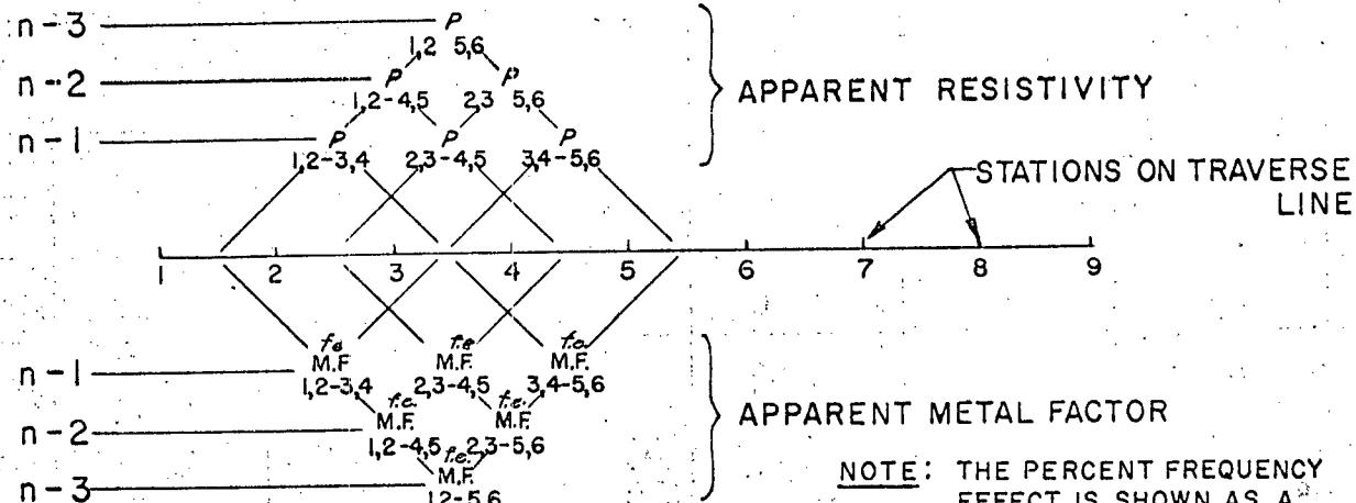
DIAGRAM SHOWING PLOTTING METHOD
