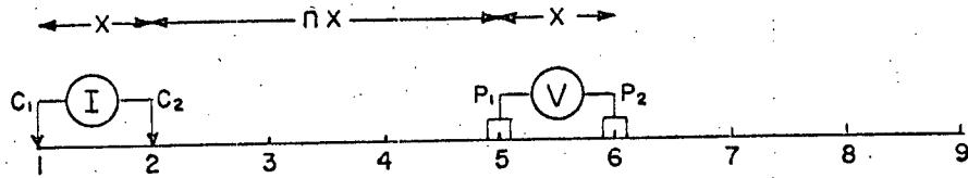
X = ELECTRODE SPREAD LENGTH OR ELECTRODE SPACING OR DIPOLE LENGTH
