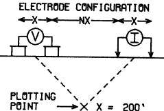
INDUCED POLARIZATION AND RESISTIVITY SURVEY
