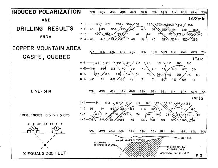
The source of the moderate magnitude IP anomaly shown in Figure 1 contains approximately 4% metallic mineralization. The zone is of limited lateral extent and enough copper is present to make the mineralization "ore grade". The presence of the surface oxidation can be seen in the fact that the apparent IP effects increase for n=2.
