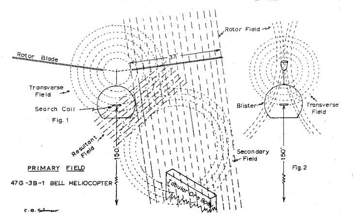
field direction that is quite different from the original and now no longer perpendicular to the axis of the search coil. Thus out of phase harmonic multiple signals are picked up in place of the secondary field.
