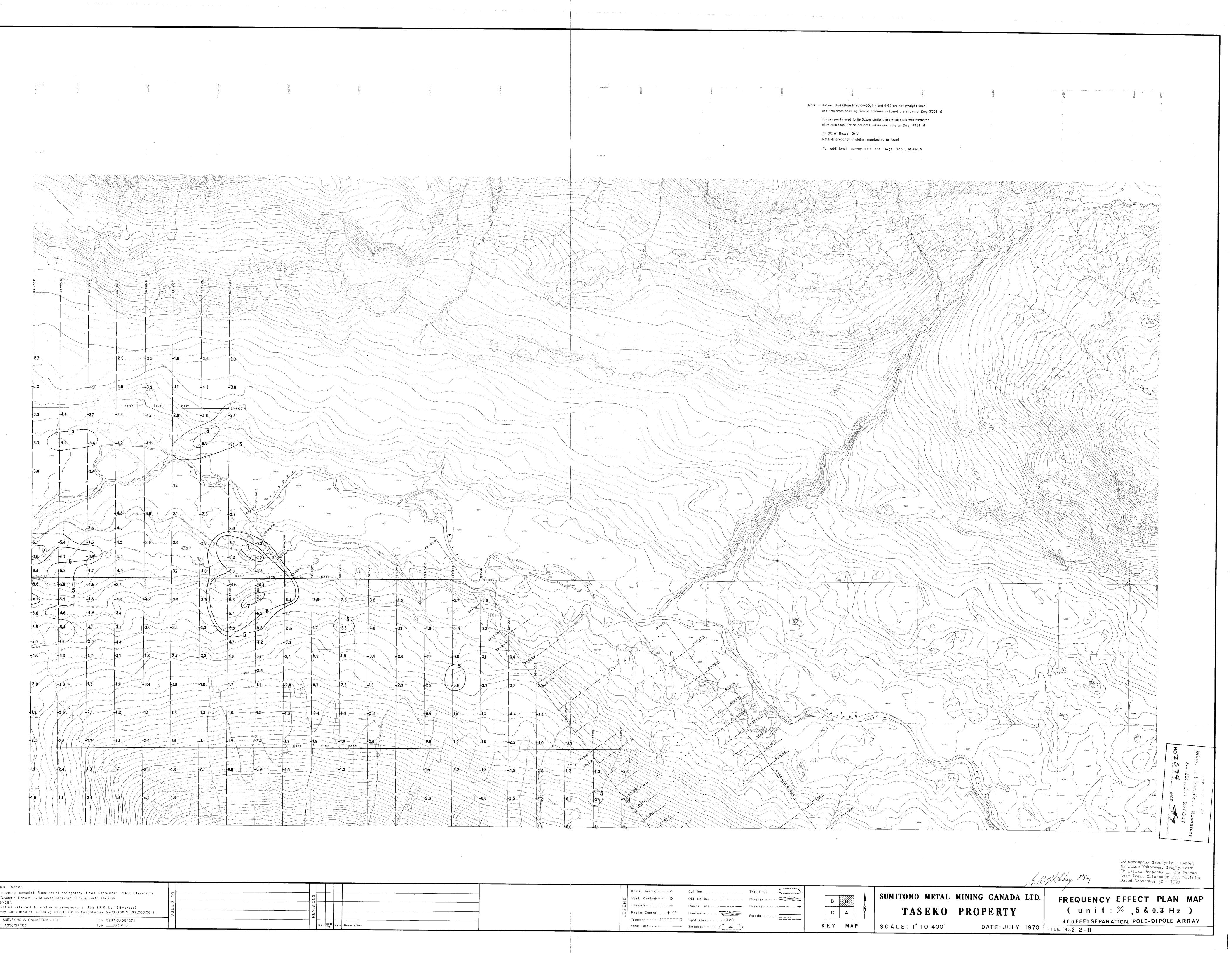
Compilation note: Topographic mapping compiled from aerial photography flown September 1969. Elevations referred to Geodetic Datum. Grid north referred to true north through meridian 123°25'. Bearing derivation referred to stellar observations at Tag SRO. No I (Empress) 1970 FP. Survey Co-ordinates 0+00 N; 0+00E = Plan Co-ordinates 99,000.00 N; 99,000.00 E. MCELHANNEY SURVEYING & ENGINEERING LTD McELHANNEY ASSOCIATES
