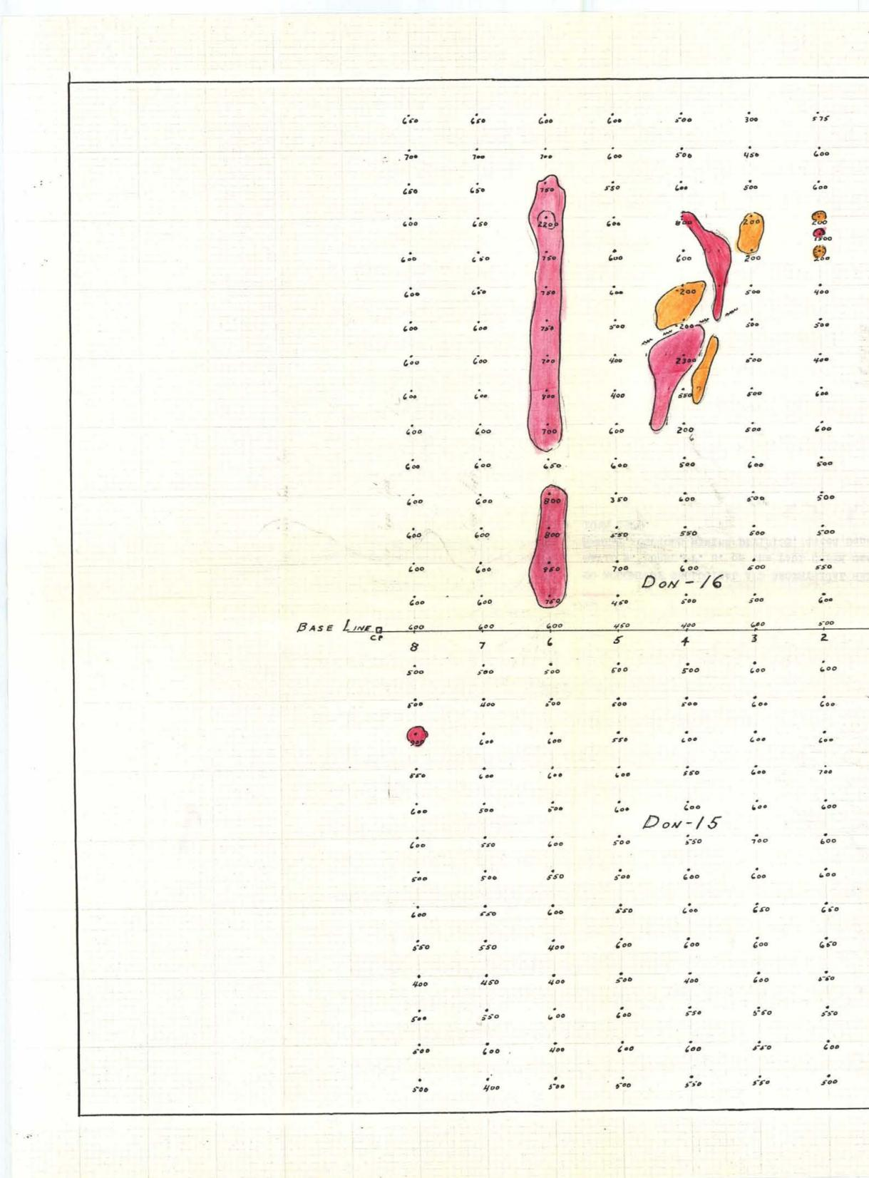
600 600 450 400 350 400 500 500 500 500 .0 400 400 600 500 \$15 H CP LEGEND 600 - RELATIVE MAGNETIC FIELD IN GAMMAS 600 . STATION LOCATION 600 MAGNETIC HIGH AREA 600 MAGNETIC LOW AREA 700 FAULT ZONE ? 600 Mines and Petroleum Resources 600 ASSESSMENT REPORT NO. 2955 MAD # 6 700 650 700 550 de Bur. CONOCO SILVER MINES LTD. (N.P.L.) 600 MAGNETOMETER SURVEY 550 DON 15-16 M.C. HEDLEY, B.C. 600 SCALE 1 - 200' Suburn DEC-1970
