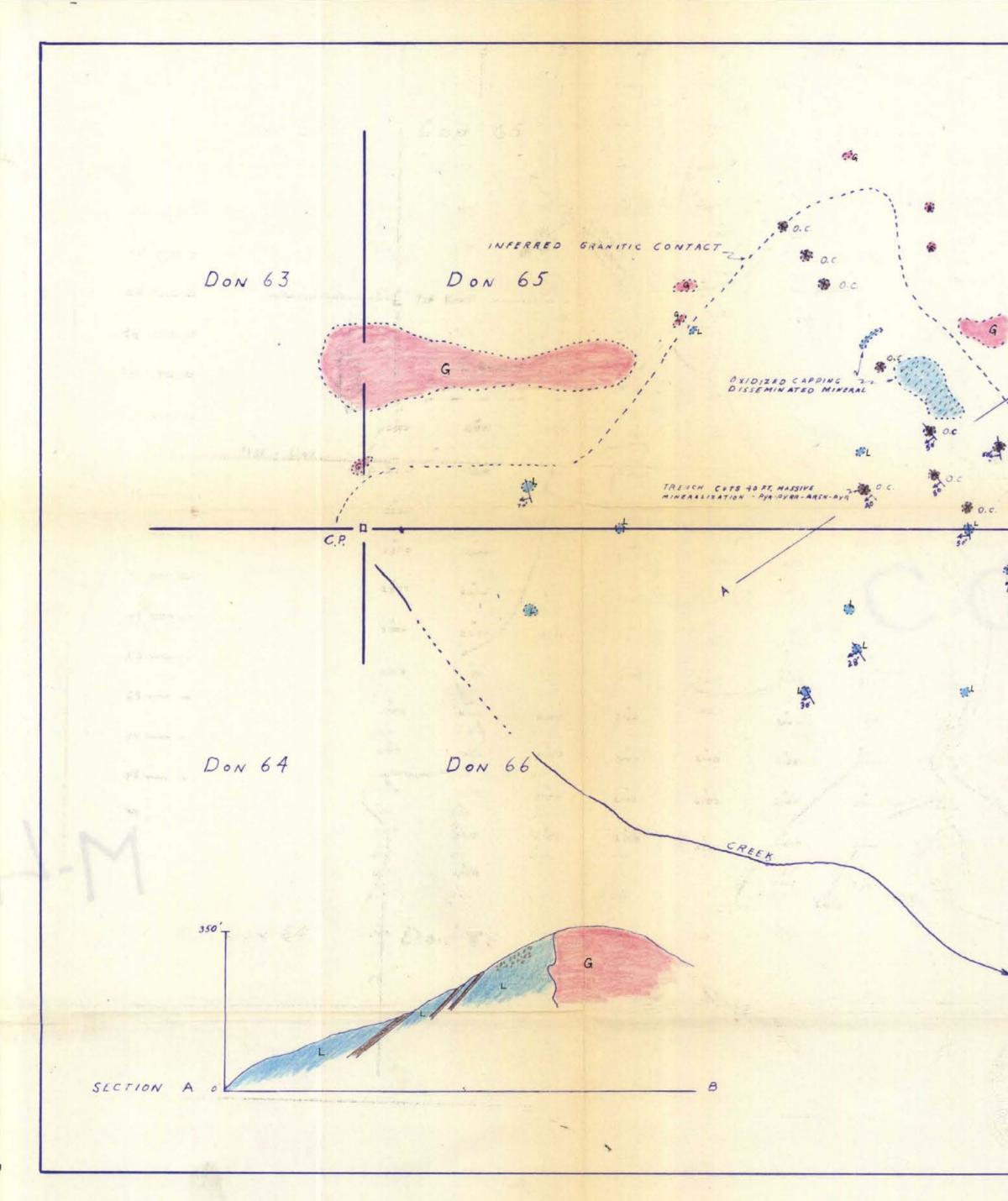
Nines and Petroleum Resources ASSESSMENT REPORT 2955 MAP 4 10. 1 LEGEND G GRANITIC IN TRUSINE BO.C. OPEN-CUT INTERSECTING BEDDING REPLACEMENT G OF LSTE. BY PYR-PYRR- ARSN'PYR. SILICIFIED LIMESTONE L Q XIDIZED CAPPING BEDDING SCALL FEET CONOCO SILVER MINES LTD. (N.P.L.) GEOLOGICAL MAP DON'S 65 Y66 M.C.S - PAUL CREEK SCALE ("= 200' Ju Burno DEC-1970
