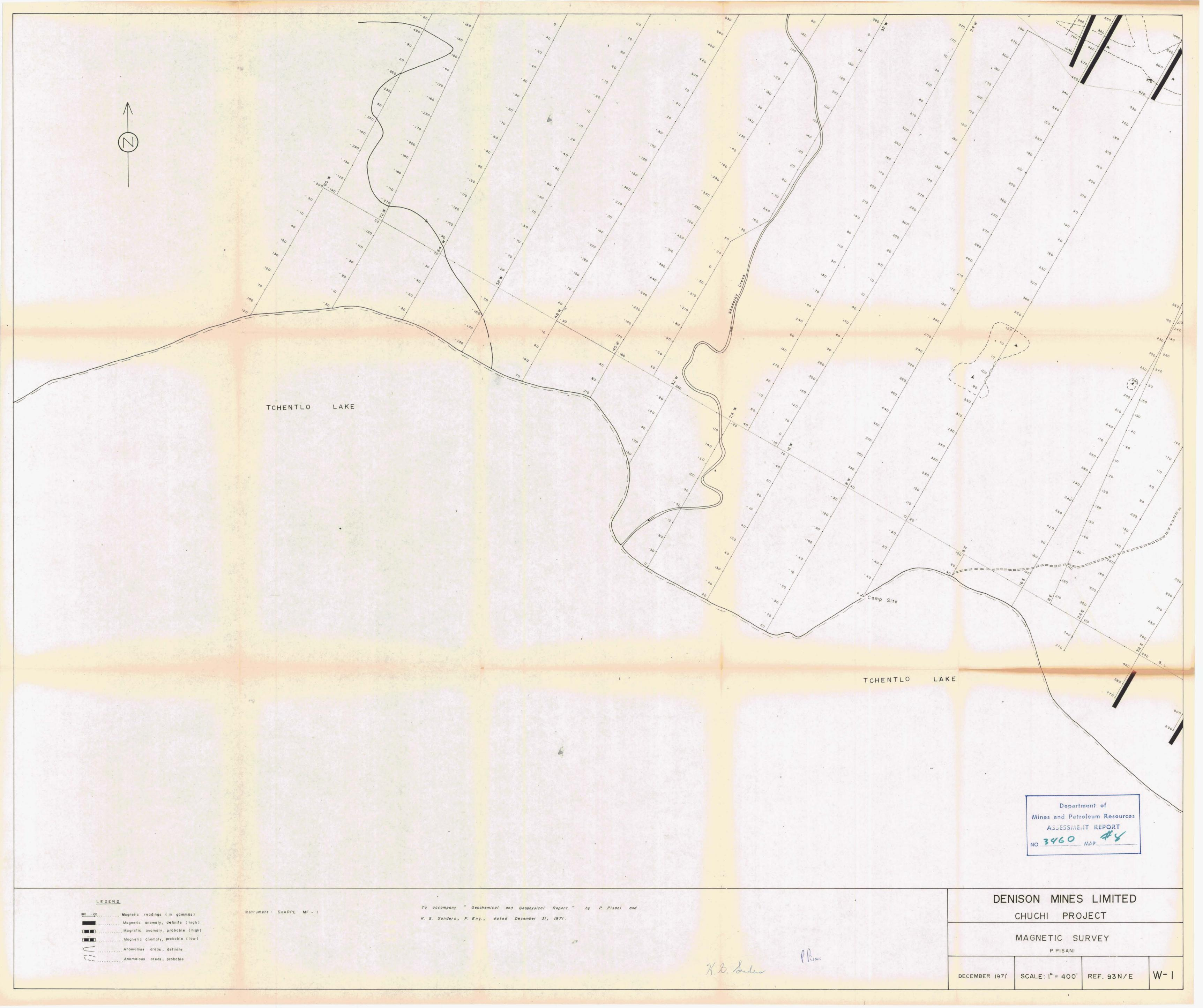
Mines and Portolaum-Resources DENISON MINES LIMITED LEGEND To accompany " Geochemical and Geophysical Report " by P. Pisani and CHUCHI PROJECT Instrument: SHARPE MF - I 180 -20 ..... Magnetic readings (in gammas) K. G. Sanders, P. Eng., dated December 31, 1971 . Magnetic anomaly, definite (high) . Magnetic anomaly, probable (high) MAGNETIC SURVEY . Magnetic anomaly, probable ( low) P. PISANI . Anomalous areas, definite . Anomalous areas, probable W-2 DECEMBER 1971 | SCALE: | = 400 | REF. 93N/E
