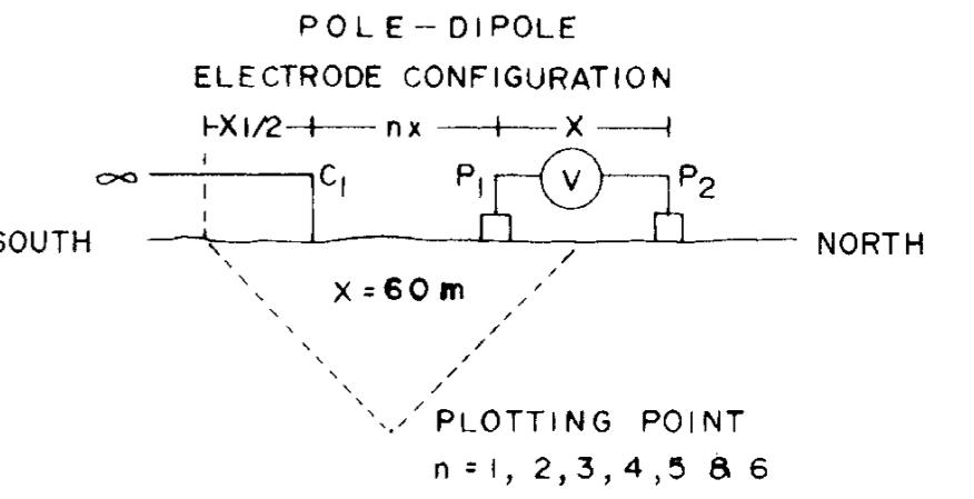
CURRENT ELECTRODE SOUTH OF POTENTIAL DIPOLE
