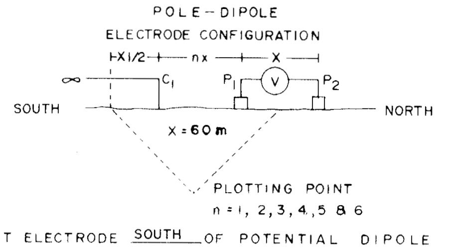
CURRENT ELECTRODE SOUTH OF POTENTIAL DIPOLEDATE SURVEYED JUNE 3, 1978
