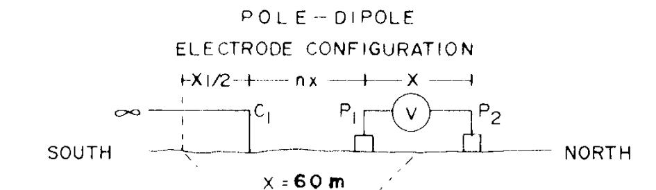
CURRENT ELECTRODE SOUTH OF POTENTIAL DIPOLE
