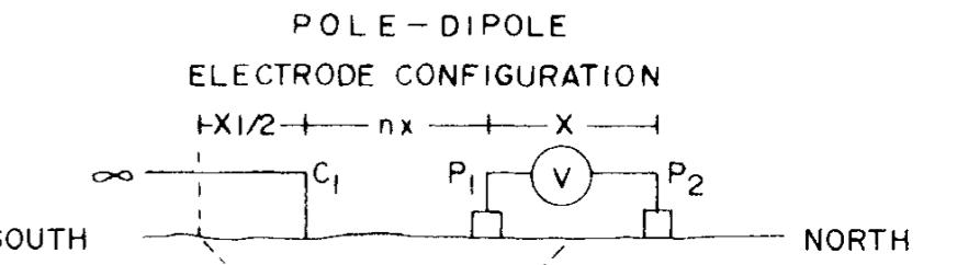
CURRENT ELECTRODE SOUTH OF POTENTIAL DIPOLE
