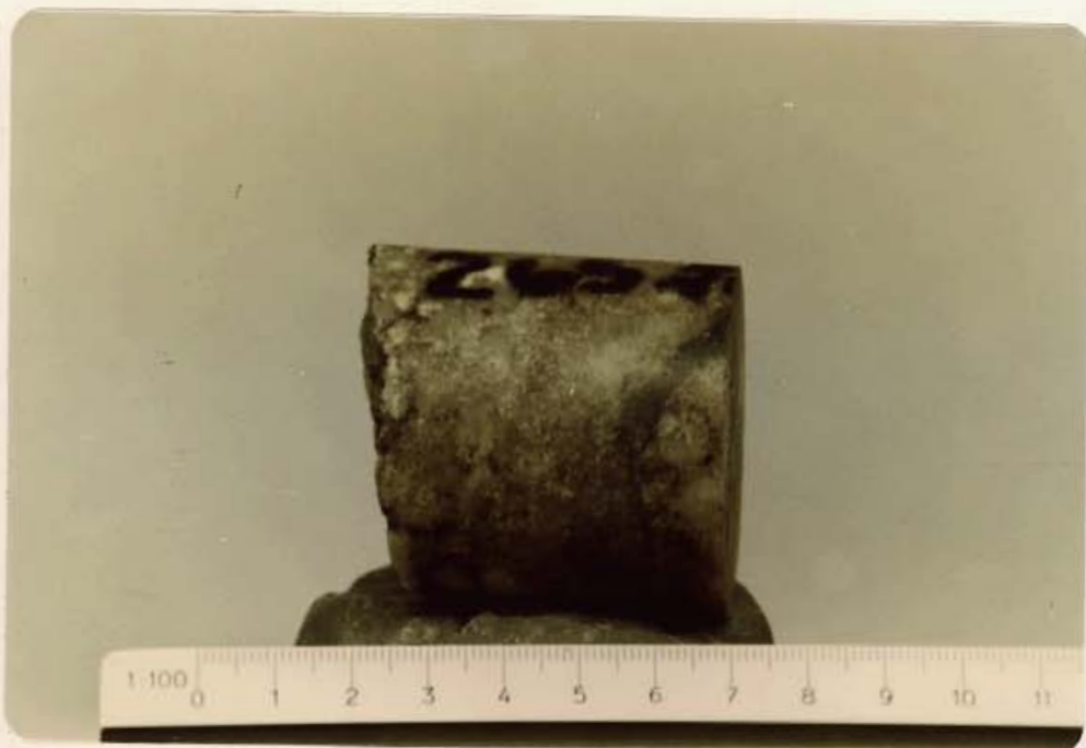
PLATE XII. Disseminated MoS 2 in siliceous section of sericite-quartz-pyrite altered Battle Porphyry.
