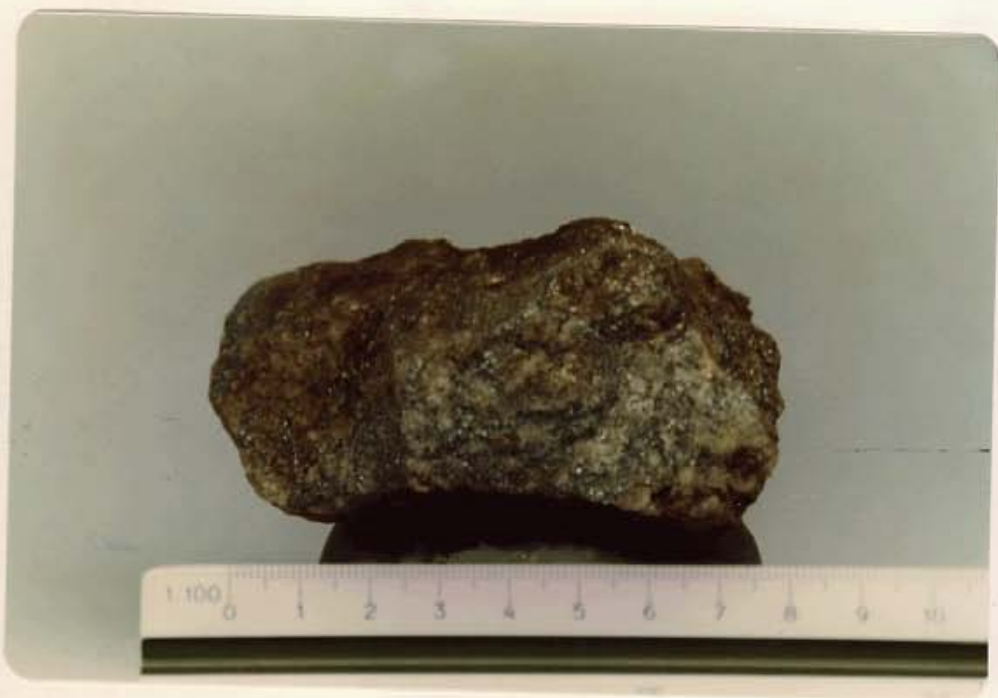
PLATE XIV. Mineralized siliceous sericite-quartz-pyrite altered Battle Porphyry from face between east and west glaciers.
