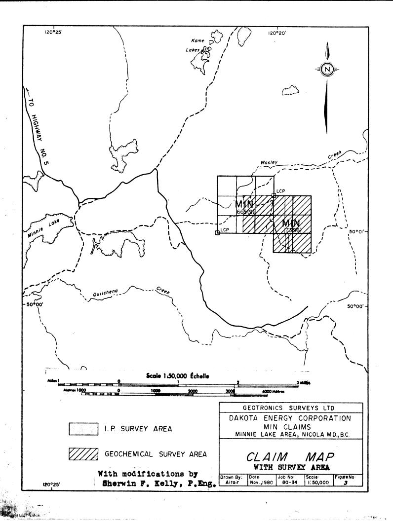
the 6-unit claims. The stations were numbered north and south from the B.L., the lines extending 500 m north and 500 m south. The B.L. was 900 m long, nine lines being run off it.
