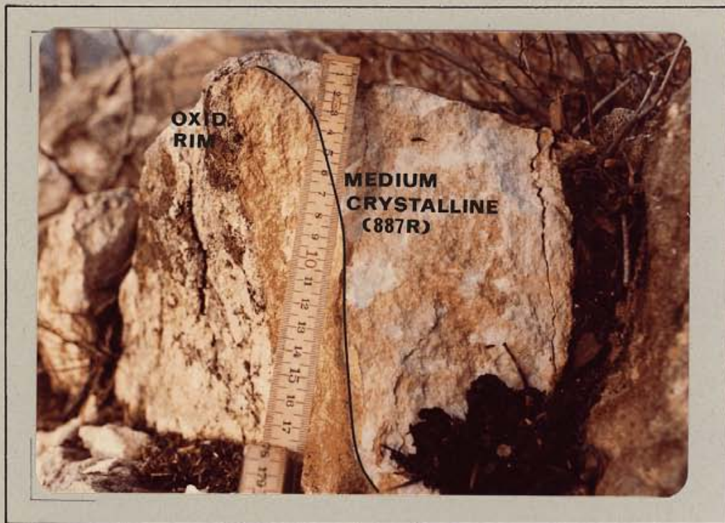
- magnesite at Station F8 . Shows surface oxidation up to 5 mm, crystal size 1 mm, massive, mottled texture. Representative material of Sample 877R .
