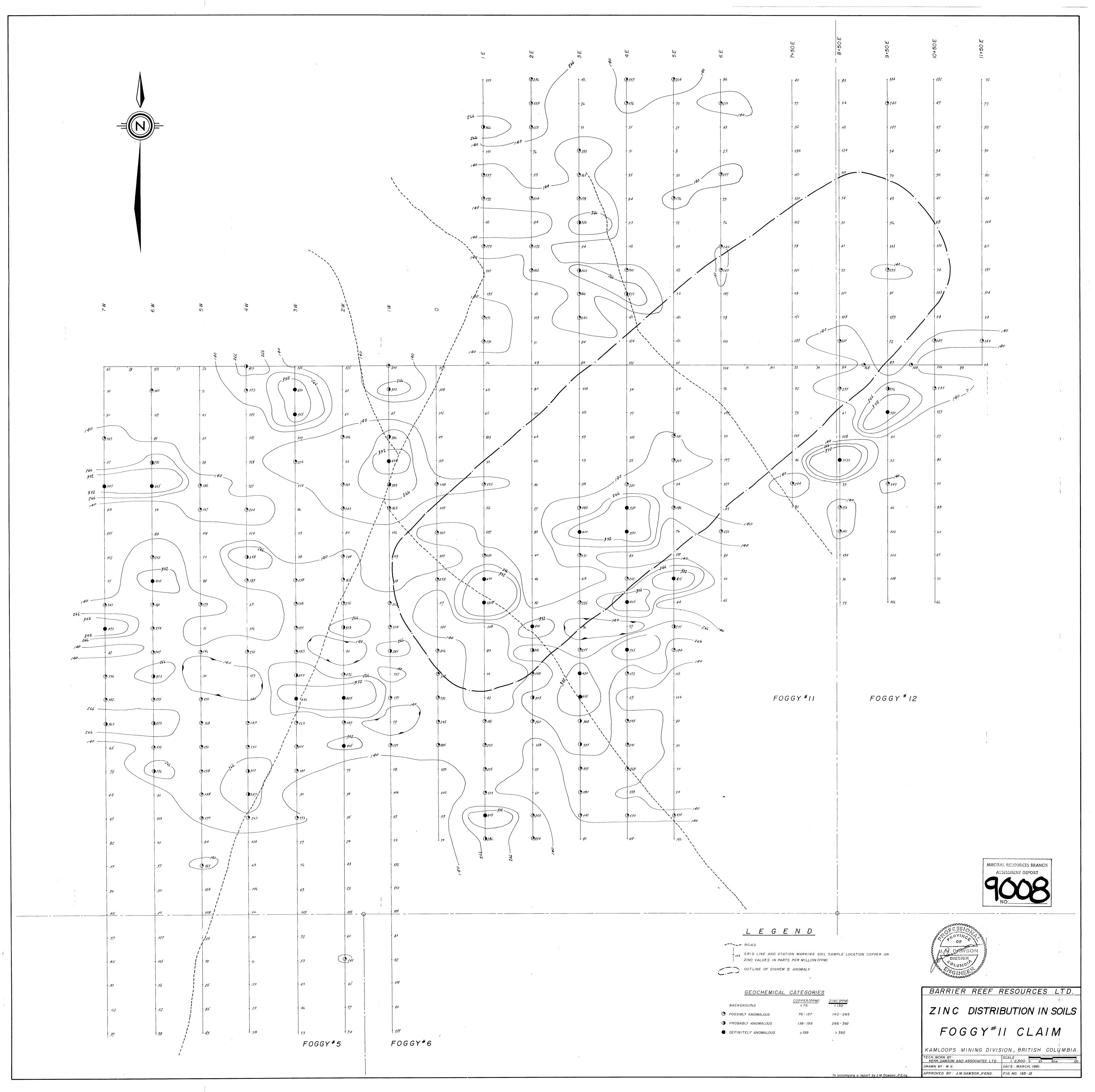
EASTERN BOUNDARY OF FOGGY II CLAIM FOGGY # 12 FOGGY #11 MINERAL RESOURCES BRANCH LEGEND ---- ROAD GRID LINE AND STATION C. ... OUTLINE OF DIGHEM II ANOMALY -8 -7 -8 GRID LINE STATION READINGS AT 25 m INTERVALS
