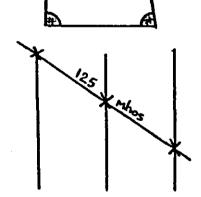
Conductor axis located by crossover anomalies with a conductance determination. The conductance is the interpreted conductivity x thickness of the conductor in mhos (same as Siemens).
