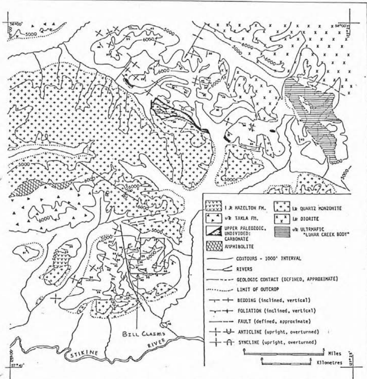
Figure 23.2. Geologic sketch map showing distribution and major structural elements of Upper Paleozoic rocks and relations to other rocks in the northwest Toadogone map area.
