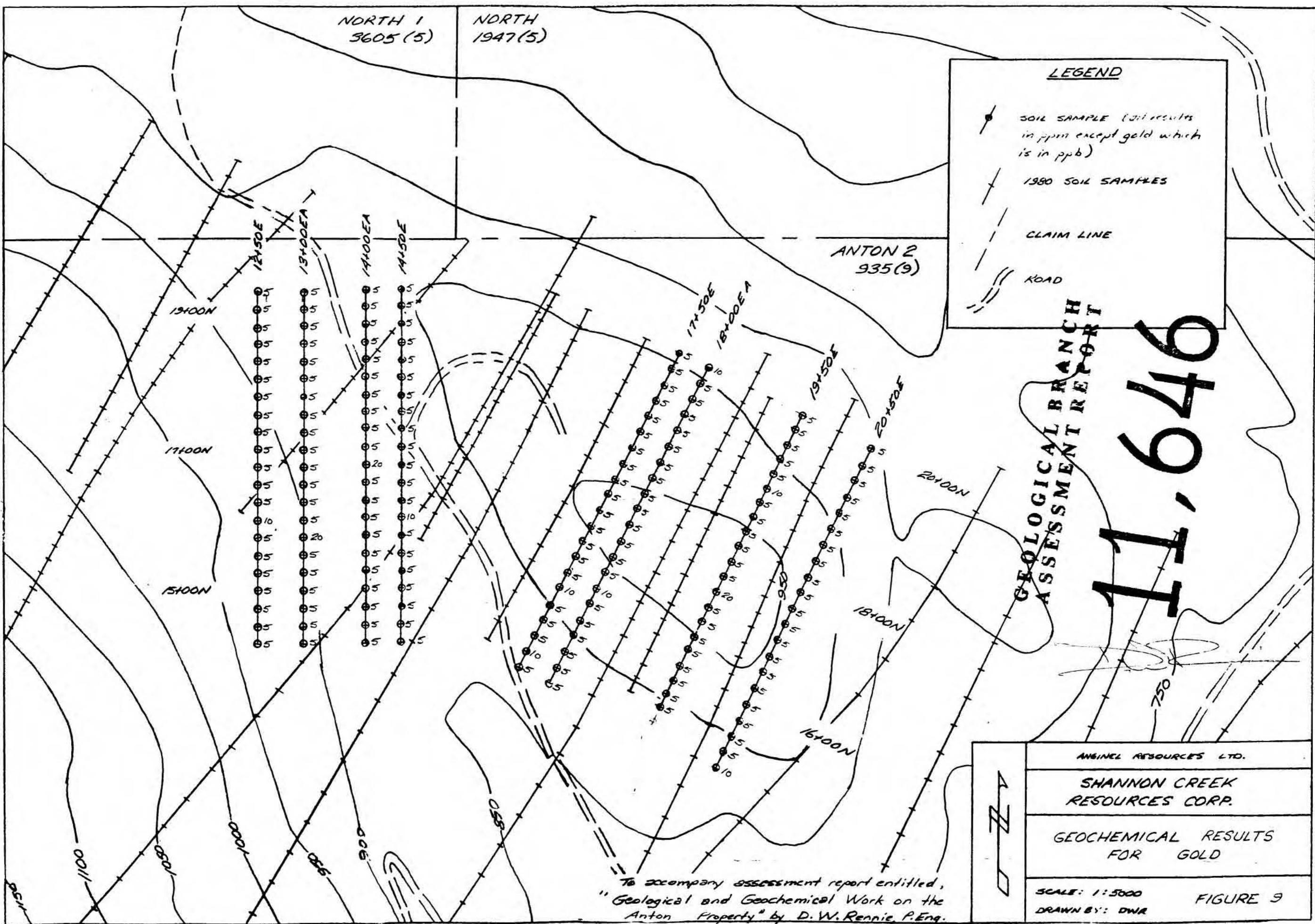
Extensions to known anomalies are not evident in the detail sampling. The "main" anomaly, which has been trenched, was detected on line 17+50E and appears to stop there. Along strike, to the southeast, on line 19+50E, an anomaly is evident and may represent the same zone.
