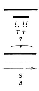
Lineation produced from magnetic and E.M. results suggesting geological structure. VLF-EM anomaly. **!, !!** Strong, extra strong anomaly. T + Terrain anomaly with a conductor anomaly superimposed. Questionable anomaly. Magnetic depression. Property boundary. ---- Claim boundary. ------ Flight line, direction flown. Seattle. Annapolis.
