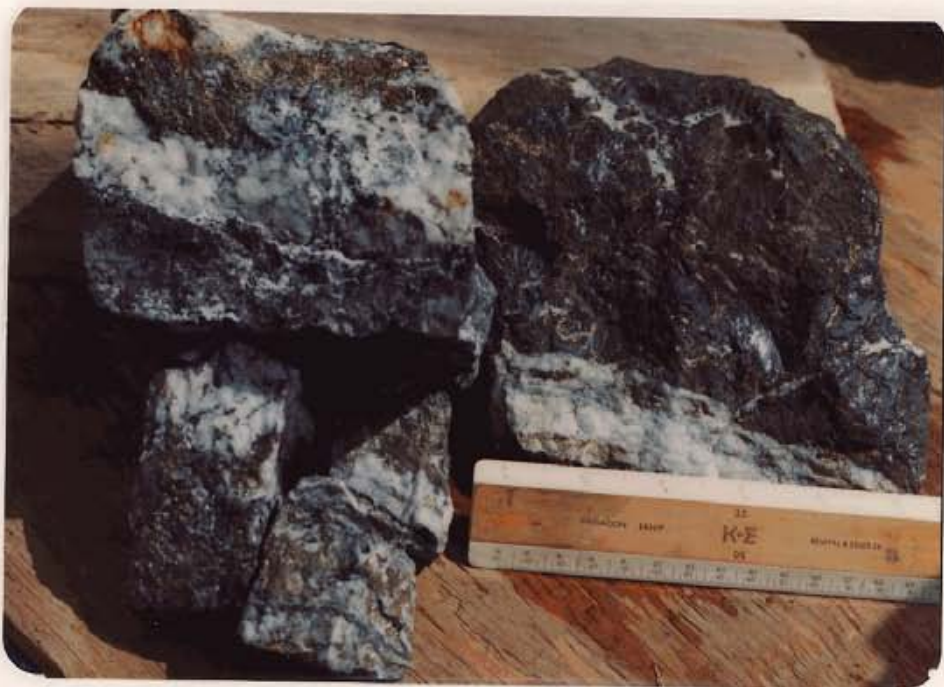
Fig. 4 Photograph of typical high grade ore consisting of quartz vein material with pyrite, galena, sphalerite, and tetrahedrite which is gold and silver bearing.
