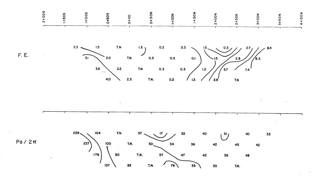
DIPOLE - DIPOLE ARRAY
