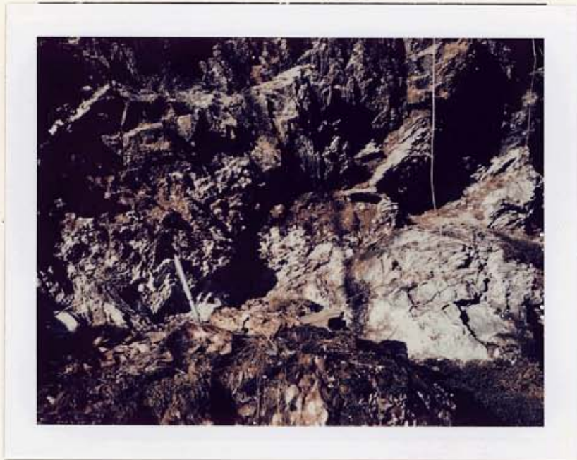
Plate 4: Post F_1 thrust fault and associated late fold (left of pencil). Quartz vein filling fault plane
