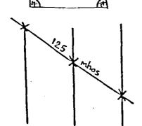
Conductor axis located by crossover anomalies with a conductance determination. The conductance is the interpreted conductivity  $\mathbf{x}$  thickness of the conductor in mhos (same as Siemens).
