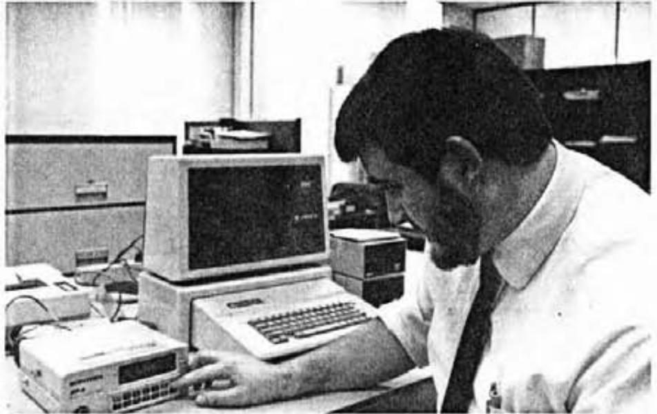
The MP-3 can be interfaced to computers such as the Apple IIe, IBMPC, Apple III, Osborne, HP-85 and others for archiving of data or further processing.
