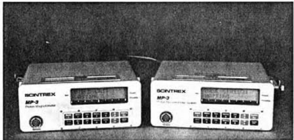
Diurnal corrections are simply made by connecting a portable MP-3 to another MP-3 which has been used as a base station.
