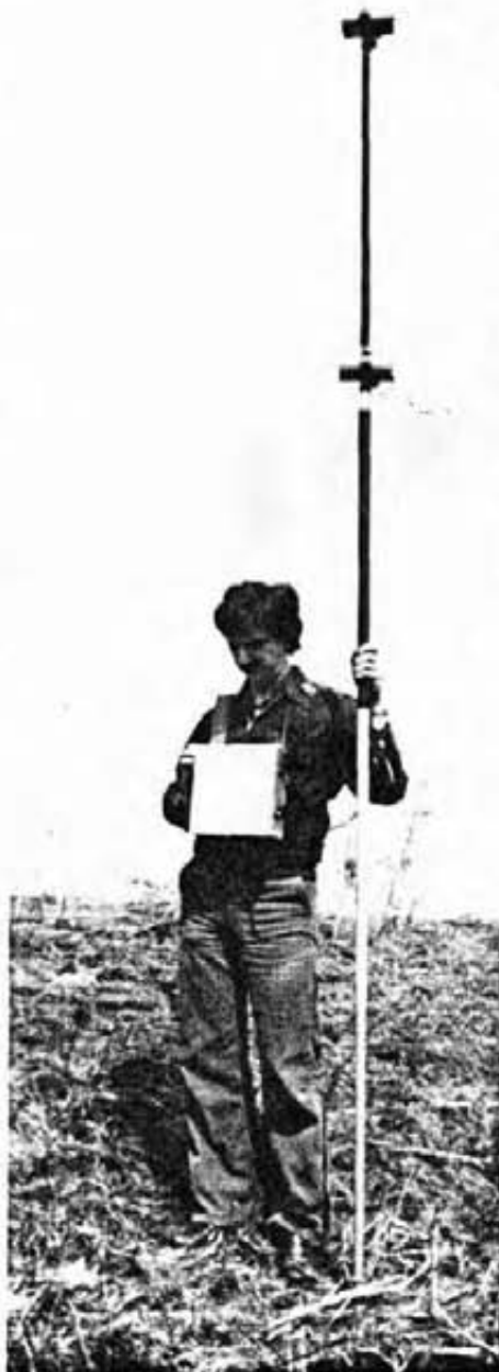
The vertical gradient measurement is made by adding a staff extender and a second sensor identical to the total field sensor.
