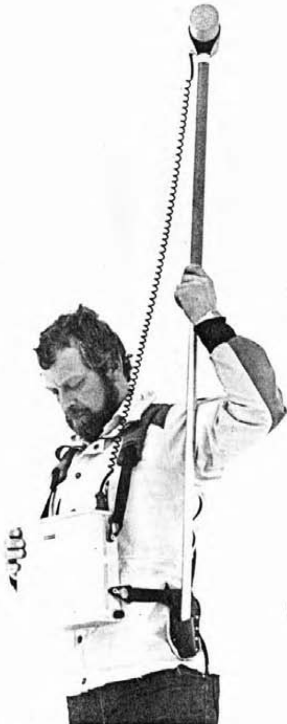
Total field measurement using staff and pouch on belt. Staff may also be extended and planted on the ground.
