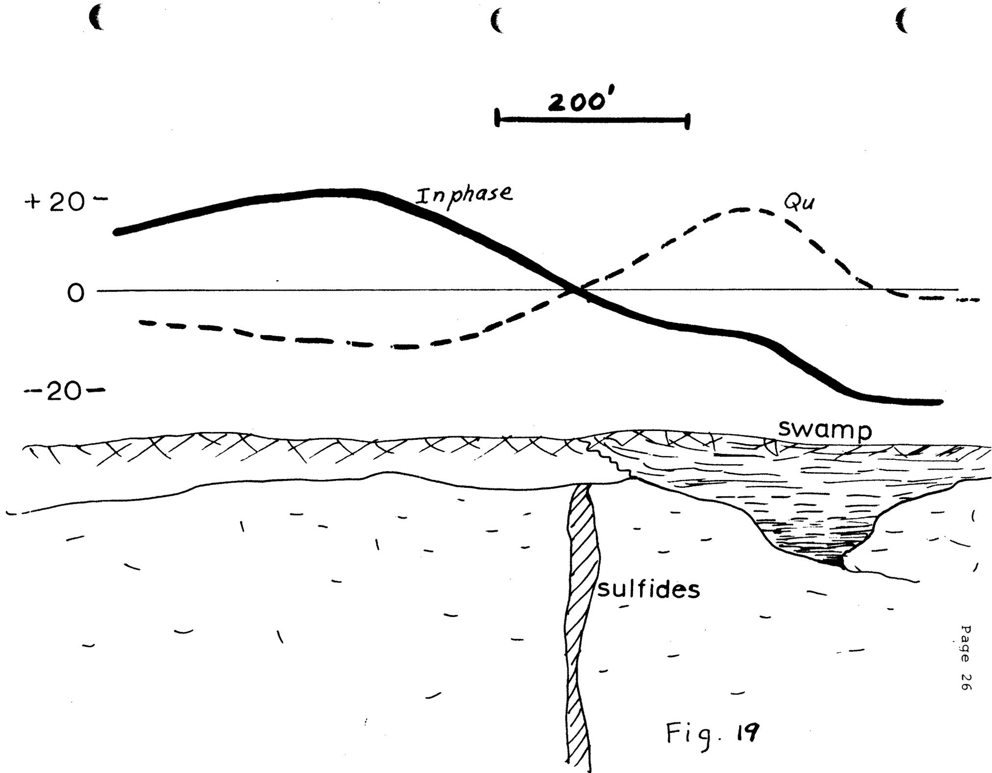
Another use for the quadrature polarity is in the tracing of a fault or a shear zone. Normally these weak conductors give a fair amount of positive (the quadrature follows the in-phase polarity) quadrature. When we have a local sulfide concentration in these structures, we get a negative quadrature response.
