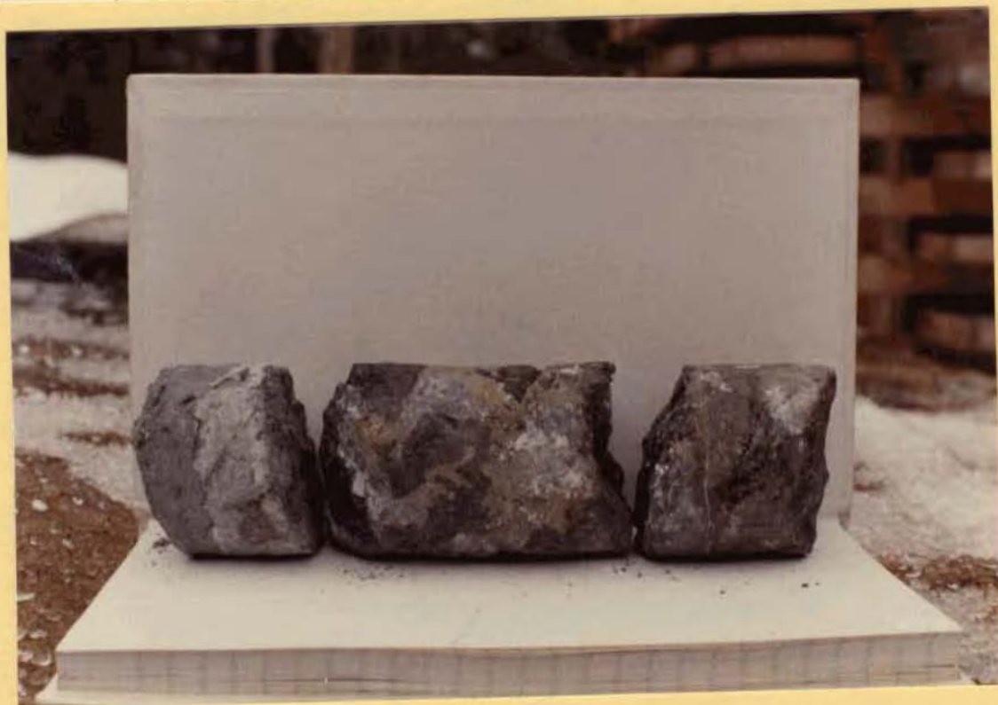
PHOTOGRAPH 2 : MASSIVE SULFIDE SECTION FROM HOLE 84-1, 98.3m - 98.6m.
