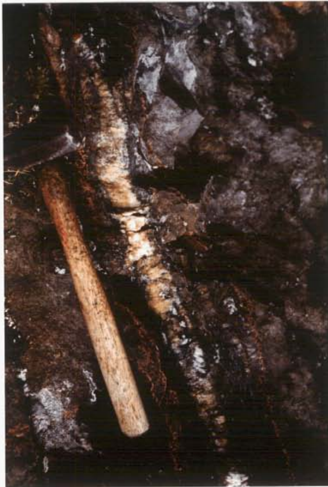
Cross-cutting quartz-oligoclase-tourmaline veinlet in dolomitic limestone. Red crayon marks the extent of scheelite mineralization. A 2m chip along the strike of the veinlet assayed 0.365% WO_3 (sample 7988).
