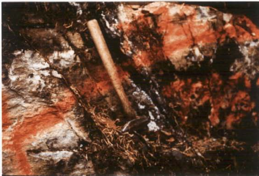
Red spray paint marks the sample width perpendicular to the fracture-controlled quartz-oligoclase-tourmaline veinlet in dolomitic limestone. This sample assayed 0.117% WO_3 over 1m (sample 7933). The skarny-altered tourmalinized rock is in lower right corner.
