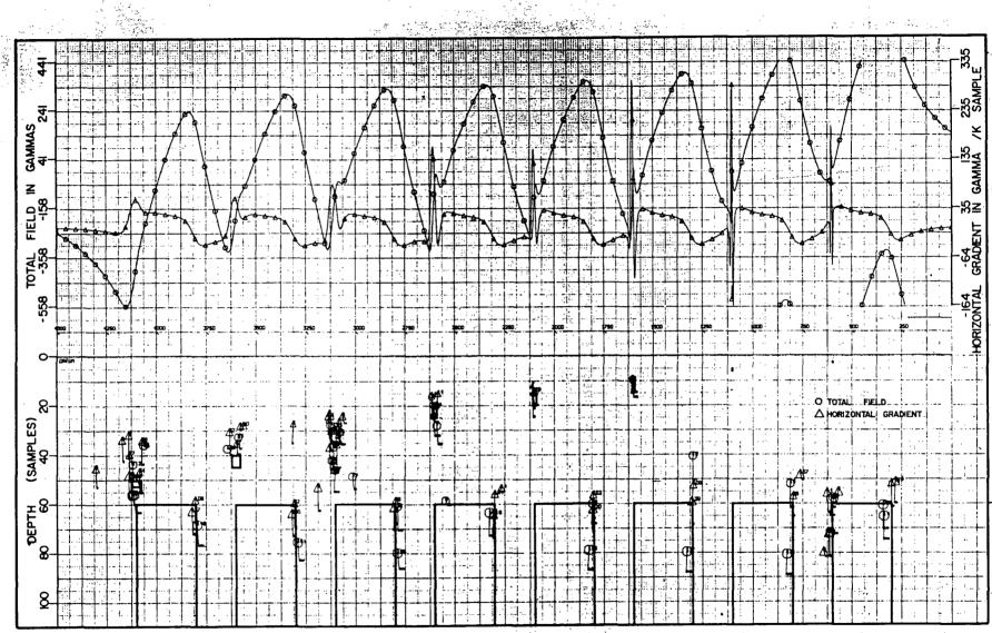
FIG. 4. Effect of shallow anomalies of moderate magnitude or deep edges.
