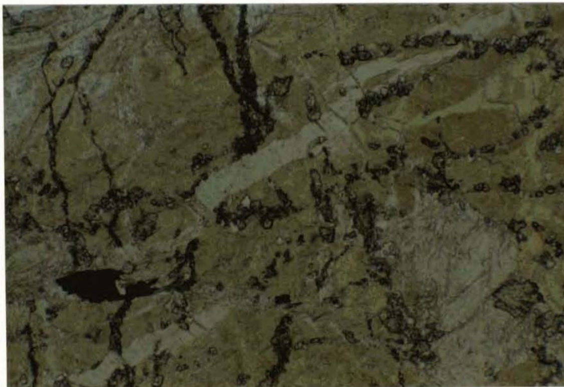
45-1 89331A. Same field as 45-0 but plane polarized light. Shows distribution of carbonate more clearly (strings of grey, high-relief granules). Antigorite is greenish brown; talc and chrysotile are light grey. Opaque oxide grain (black) at lower left.
