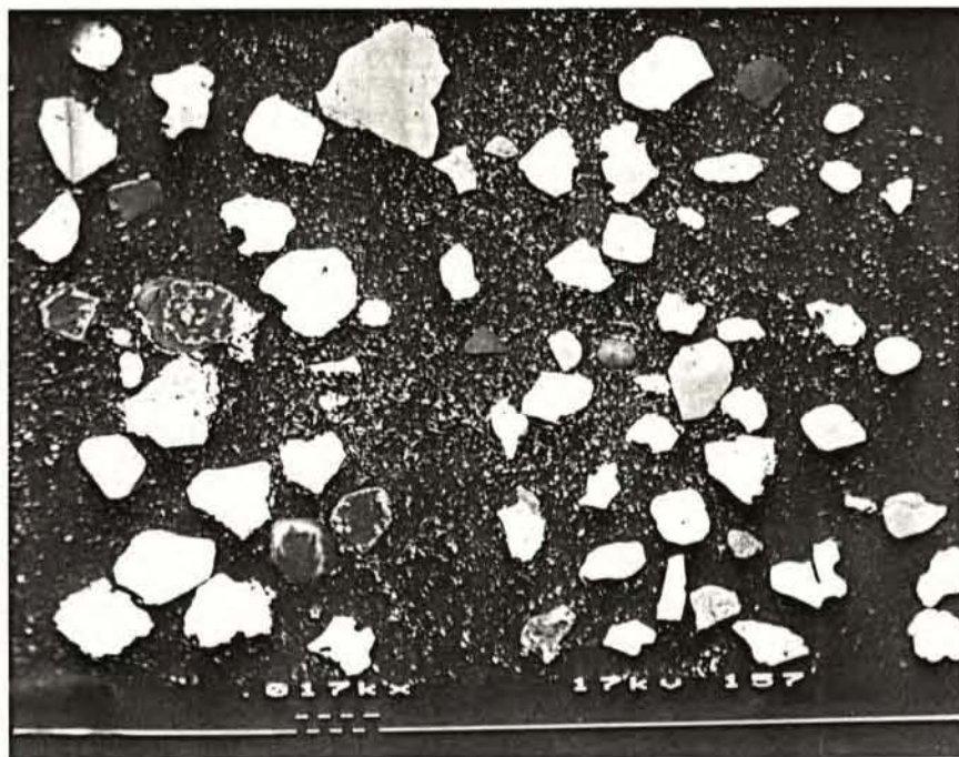
SEM area scan and photograph of ilmenites, chromites & magnetites - JACK 14B sample
