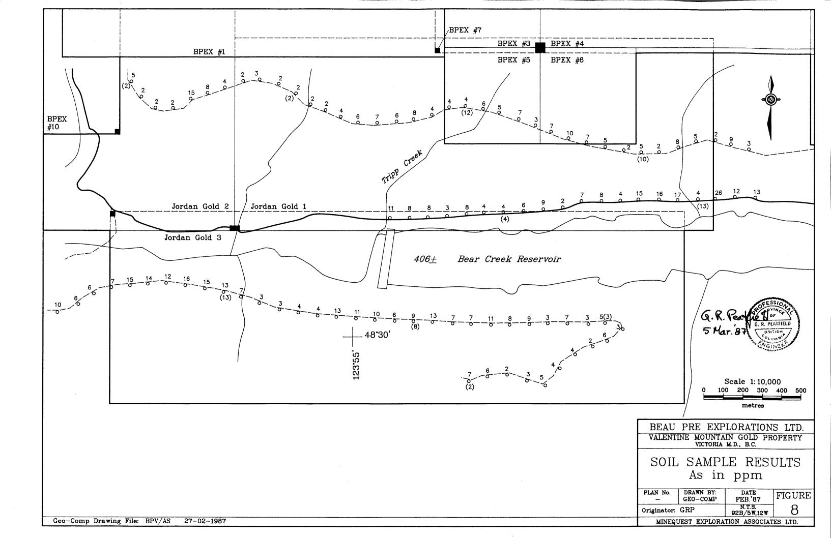
There does not seem to be a simple relationship between As and Au contents of the soil samples. Many samples with erratic high Au results returned very low As values, although there does seem to be a tendency for samples with higher As contents to have detectable amounts of Au.
