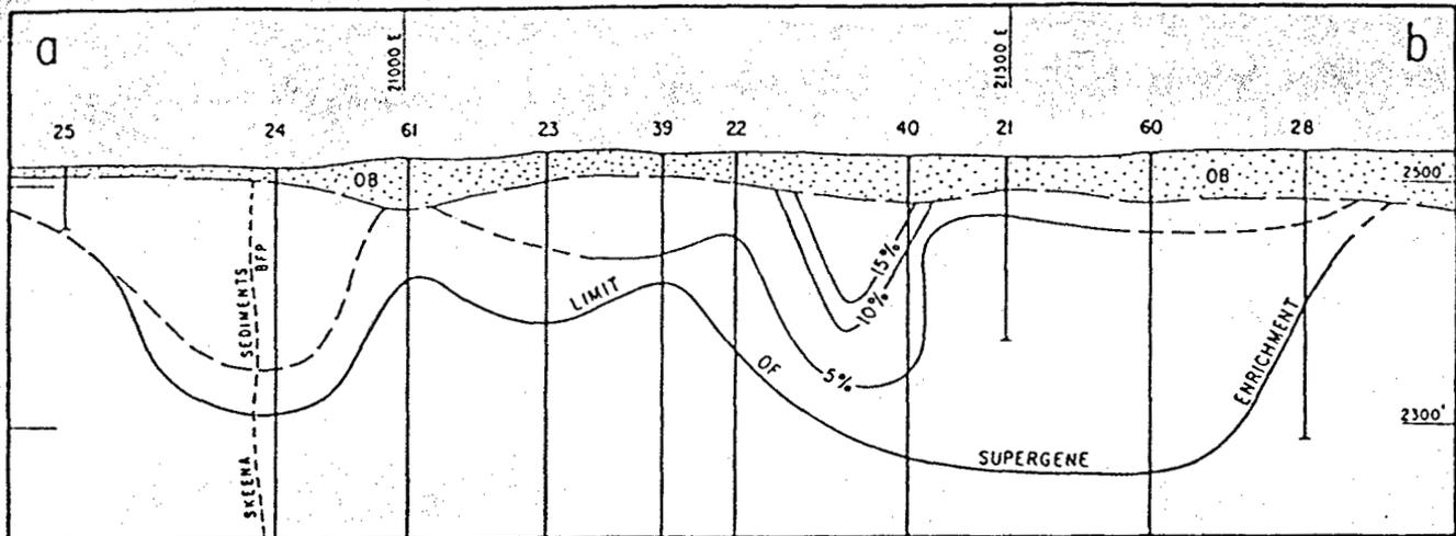
FIGURE 23—Profiles of Oxidation and Supergene Enrichment Across the Western Segment of the Bell Copper Orebody (see Fig. 9, line a-b, for location). Contours of 5%, 10% and 15% Cu oxide/total Cu are shown.
