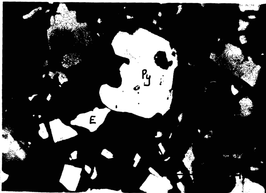
Figure 2. Lead cleaner concentrate with electrum (E) locked with sphalerite (Sp), which in turn is locked with pyrite (Py). (X666, incident light)
