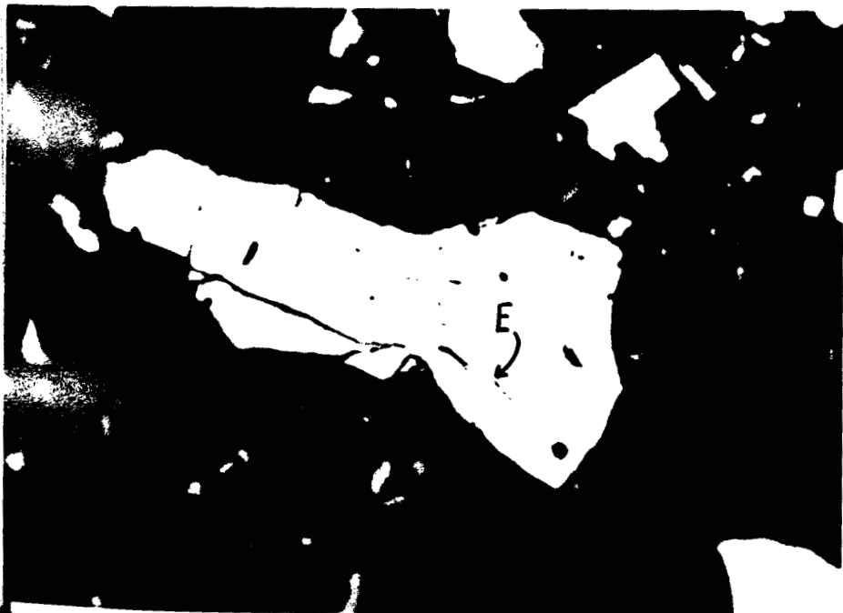
Figure 3. Lead cleaner tailing. Fine electrum (E) about 8 \mu\text{m} in length as inclusion in pyrite. (X666, incident light)
