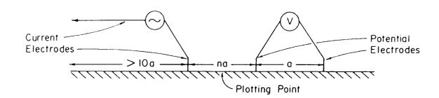
The electrode spacing (or dipole length) is denoted at 'a' and was chosen as 50 m. The 'n' was read from 1 to 3 dipole separations ('na') which was therefore 50 to 150 m. This gives a theoretical depth penetration of 75 to 100 m which depends not only on the 'na' spacing but also on the ground resistivity.
