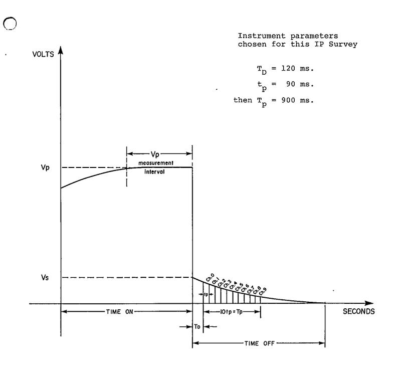
Mark IV Receiver Measurement Parameters
