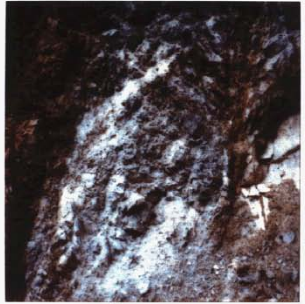
# 10 1.5m HEMATITE MYLONITE WITH MALACHITE STAIN HEMATITE HM - 1
