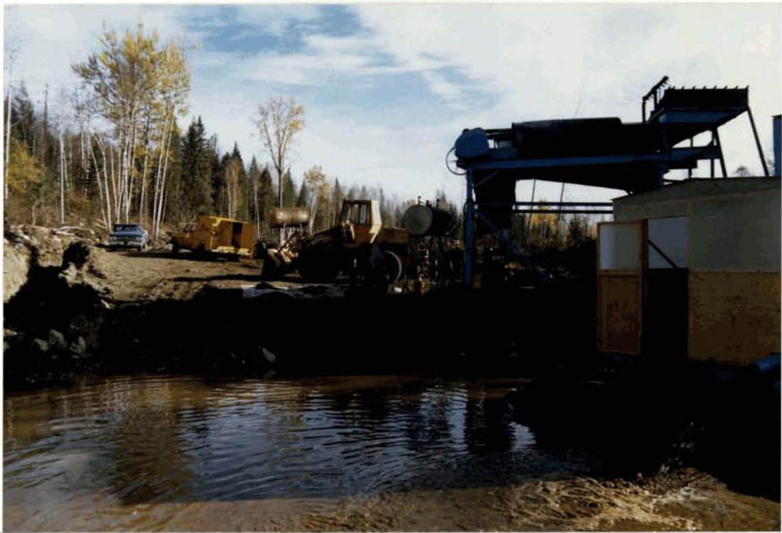
FREGOLD'S RECOVERY PLANT, DISCHARGING DIRECT TO SETTLING POND. MAINTAINING 100% RECYCLE, ZERO DISCHARGE OF WATER
