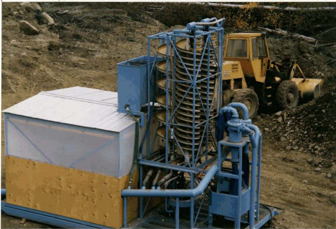
FREEGOLD'S RECOVERY PLANT, CONSISTING OF CYCLONS, MARK VII REICHERT SPIRALS AND GEMINI TABLE
