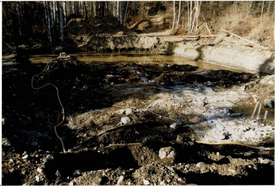
BEDROCK EXPOSURE CLEANED WITH BACKHOE, CREATING SETTLING POND AREA. MAINTAINING 100% RECYCLE, ZERO DISCHARGE OF WATER
