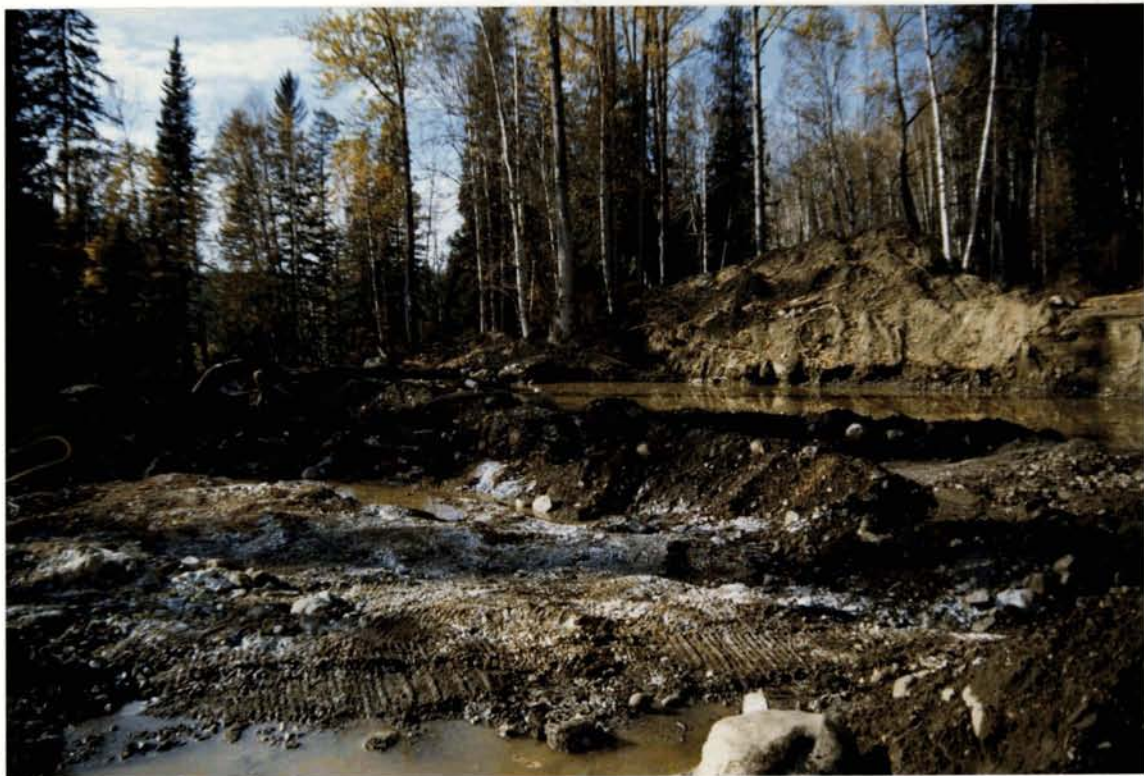
BEDROCK EXPOSURE CLEANED WITH BACKHOE, CREATING SETTLING POND AREA. MAINTAINING 100% RECYCLE, ZERO DISCHARGE OF WATER
