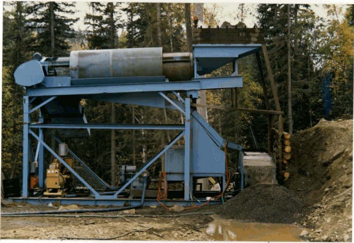
FREEGOLD'S BULK SAMPLING TROMMEL PLANT SET IN PLACE FOR FIRST BULD SAMPLING PROGRAM
