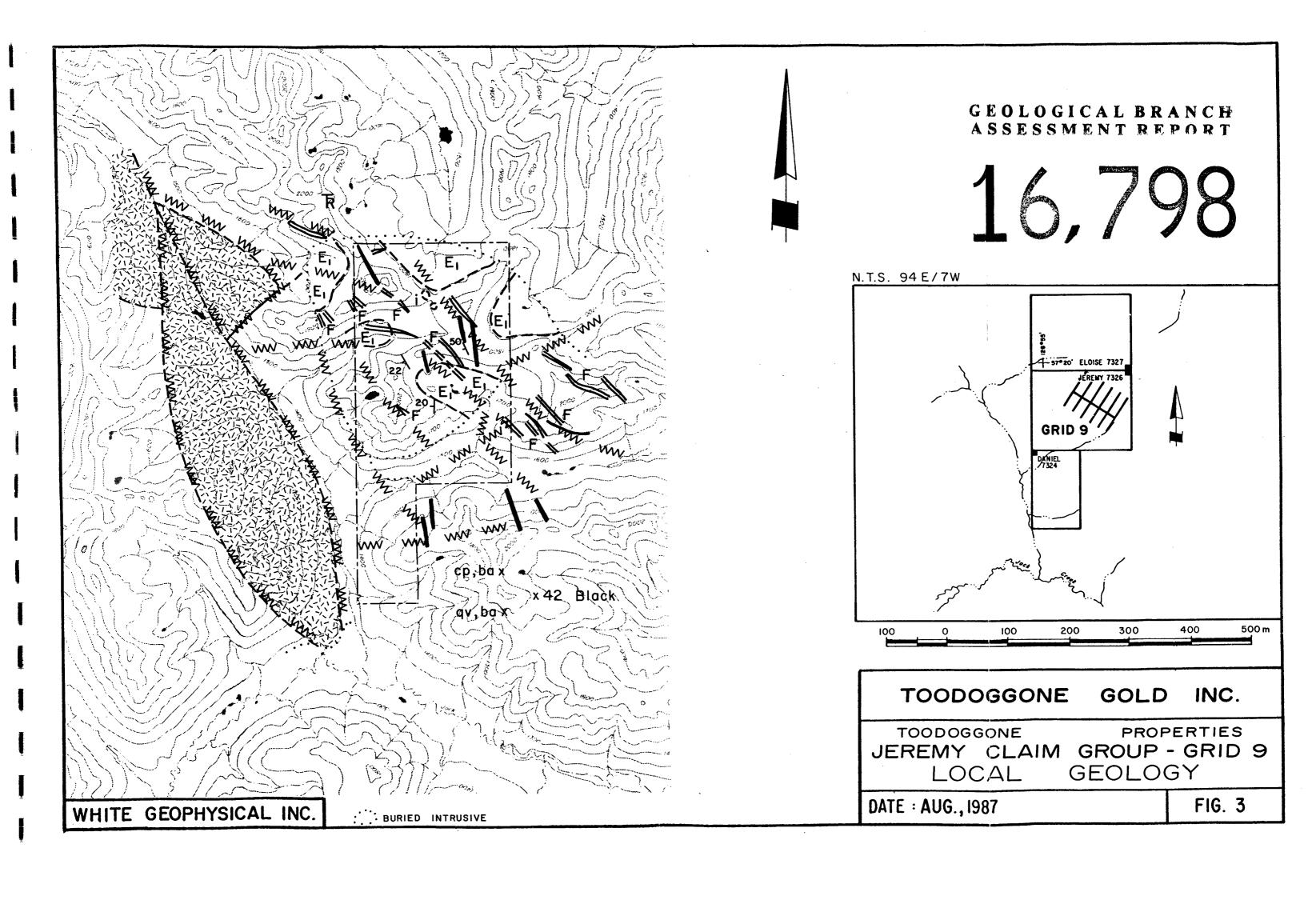
folding and faulting activity. The local geology map (Figure 3) shows an elongated intrusive on the west side of the claims area, and two crossing fault systems suggesting the presence of a lateral pressure in a west-east direction. The folding activity is evidenced in the Jeremy claim by the deformed pyroclastic formations in the area visited and staked by the writer (see Figure 4).
