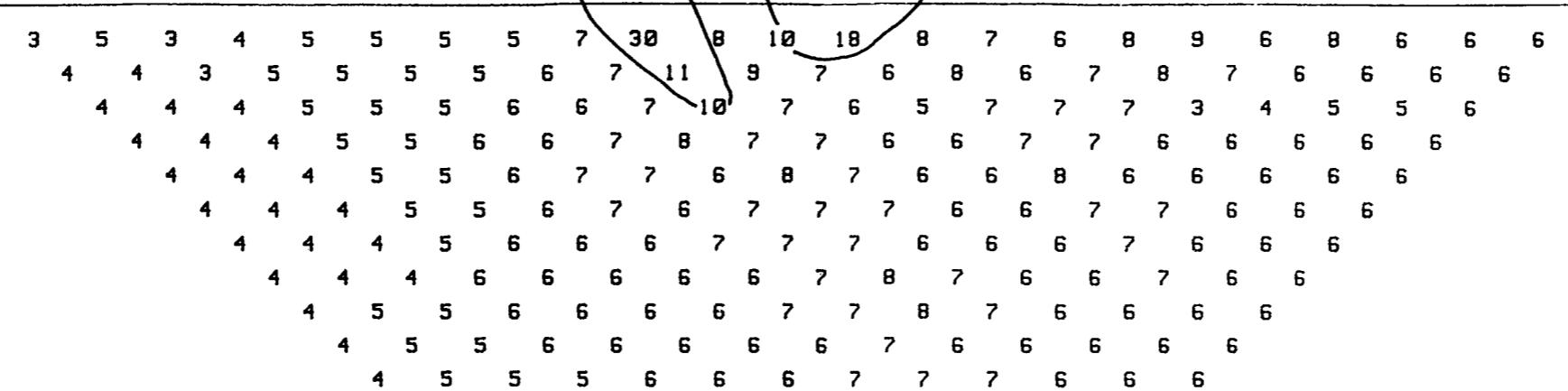
APPARENT RESISTIVITY (Ohm-metres\*10)
