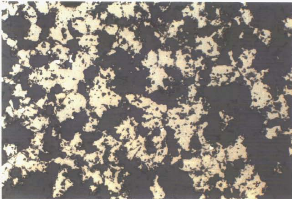
Plate 5b. Same section, reflected light. Dark grey material is quartz, light grey is sphalerite and highly reflective yellowish white grains are pyrite. Scale as above.
