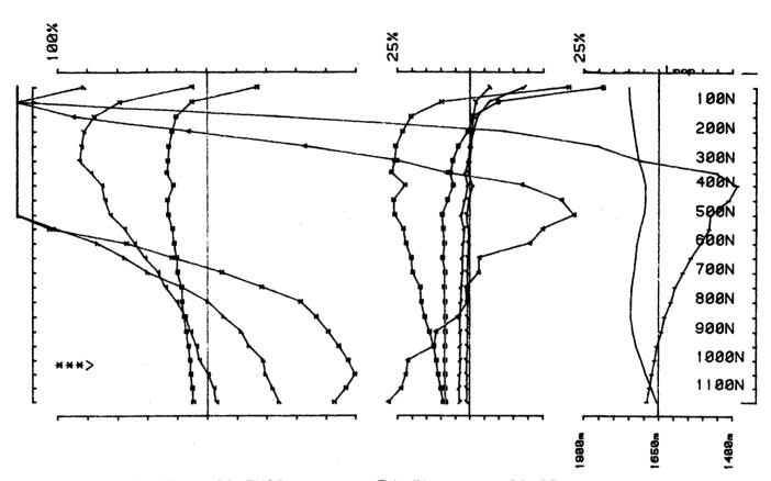
Area SHA SOUTH COMINCO operator IJ JV freq(hz) 30.974 Loopno 7 Line 10 component Hz secondary Ch 1 normalized Ch 1 reduced
