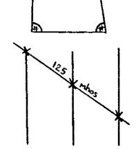
Conductor axis located by crossover anomalies with a conductance determination. The conductance is the interpreted conductivity x thickness of the conductor in mhos (same as Siemens).
