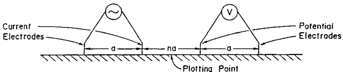
The dipole length ('a') was chosen to be 30 m. It was read to five separations ('na') which was therefore 150 m which gives a theoretical depth penetration of 75 to 100 m.
