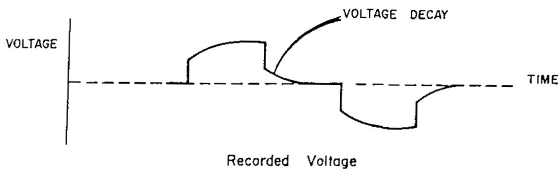
Time-domain measurements involve sampling the waveform at intervals after the current is switched off, to derive a dimensionless
