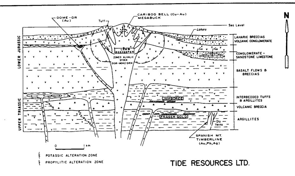
Diagrammatic Cross-section Through the Quesnel Trough Volcanic Complex, Showing Relative Stratigraphic Positions of Known Mineral Deposits
