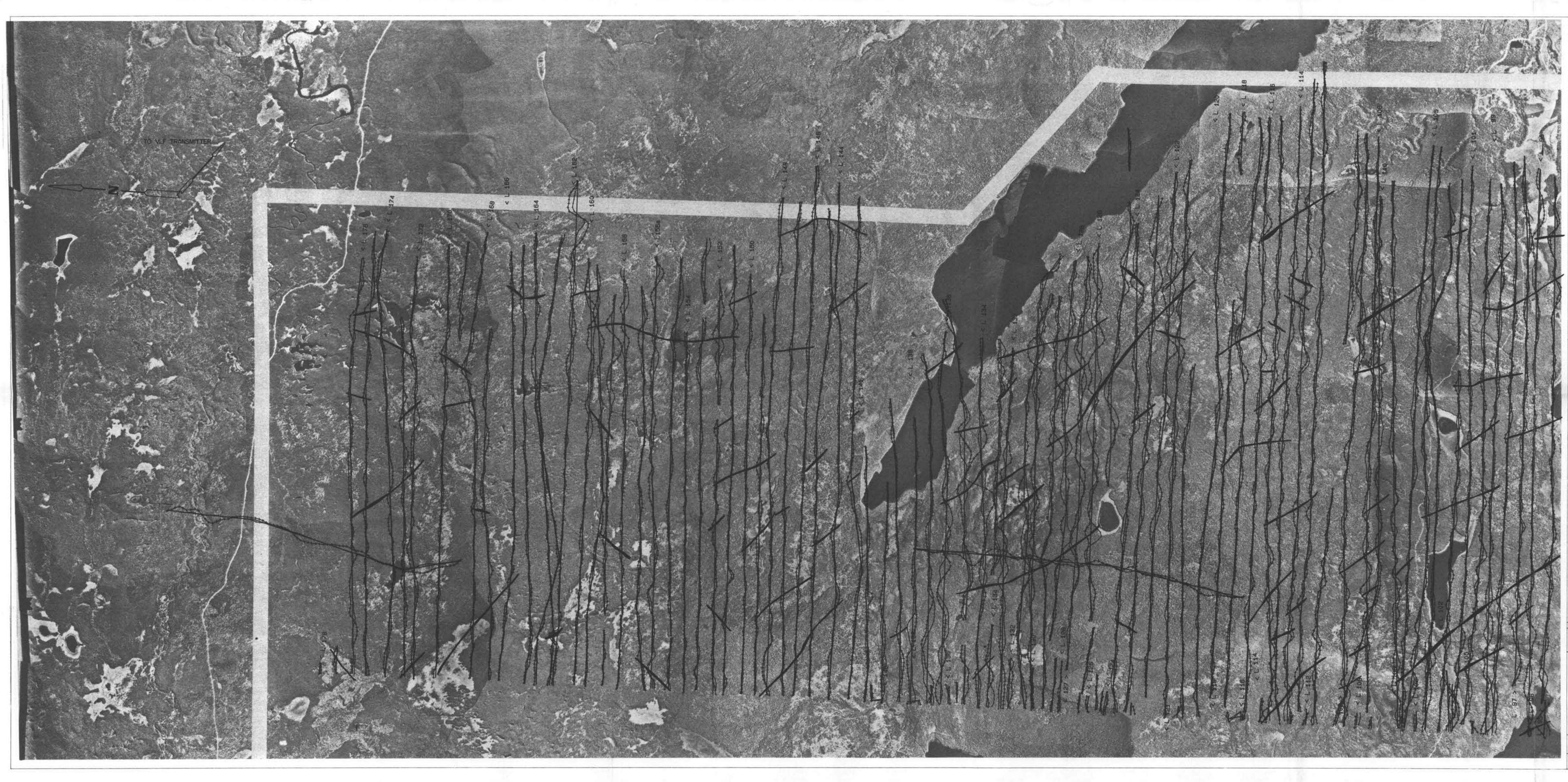
GEOLOGICAL BRANCH ASSESSMENT REPORT VLF-EM CONDUCTOR TOTAL FIELD-Base=0 Scale=25/cm QUADRATURE - Base=0 ----Scale= 25% /cm N.T.S. 93A/3W TIDE RESOURCES LTD. LAC LA HACHE PROJECT Northeast Block VLF-EM Profiles (Annapolis) Scale 1: 20000.0 Fig.9 Date: December 1988 Survey: September 1988 WESTERN GEOPHYSICAL AERO DATA LTD.
