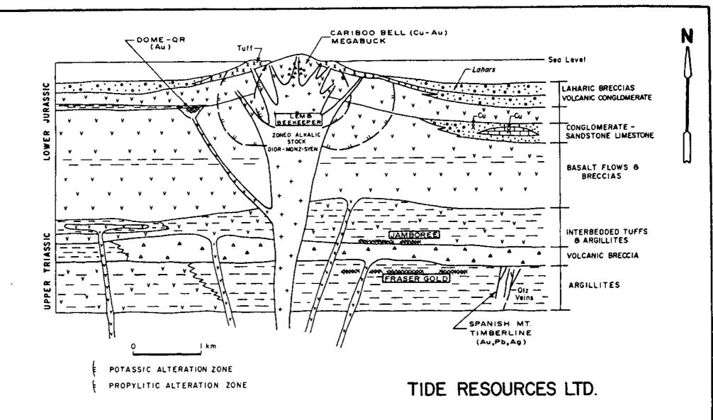
Diagrammatic Cross-section Through the Quesnel Trough Volcanic Complex, Showing Relative Stratigraphic Positions of Known Mineral Deposits Vein-hosted gold deposits where the gold mineralization has been remobilized and concentrated in quartz veins in the vicinity of stratabound deposits. These deposits form small, high-grade orebodies which, because of previous discouraging results, have a low exploration priority.
