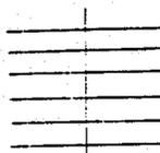
1987 Grid. Cut, chained, picketed. 100 m. spaced lines. 25 m. stations.
