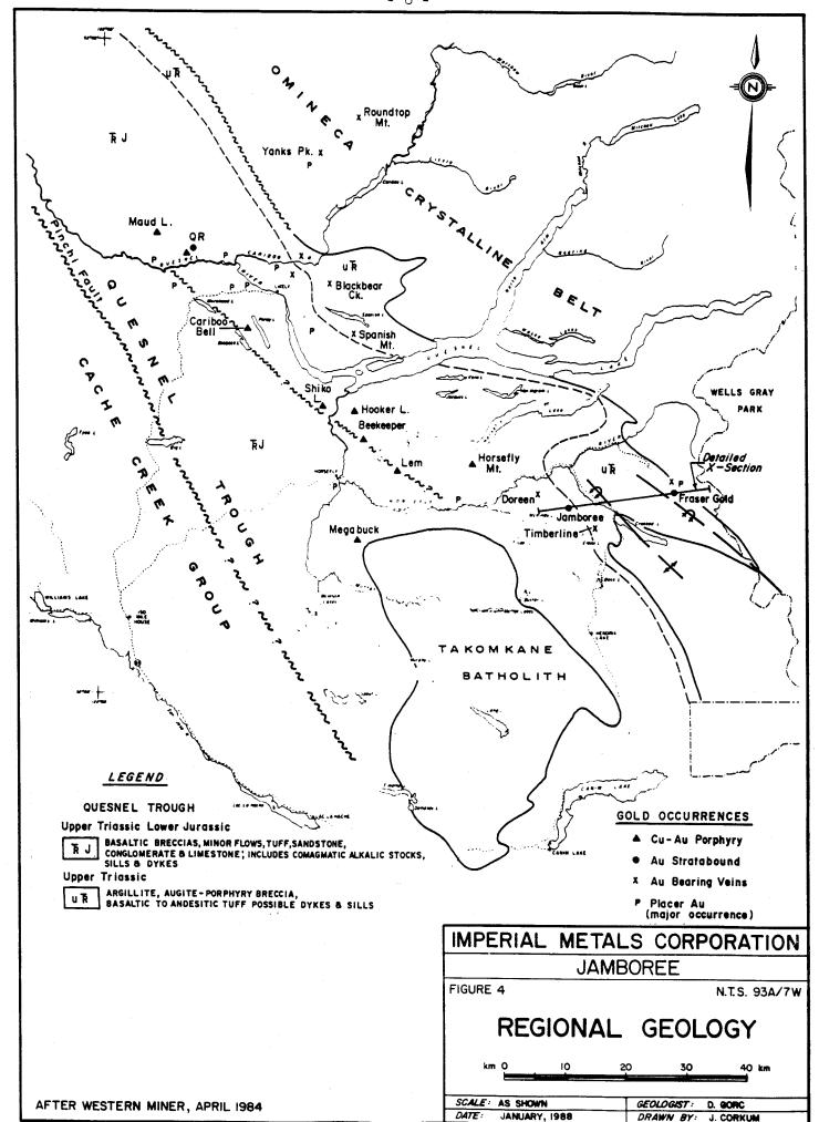
The lower part of the unit 1 assemblage is exposed near Doreen Creek and consists of interbedded and commonly laminated, argillites and tuffs. The rocks are virtually unmetamorphosed with the exception of a hornfels halo developed around a dioritic stock. Equivalent rocks exposed north of the Horsefly River are cherty tuffs overlain by laminated tuffs with occasional lapilli tuff horizons.
