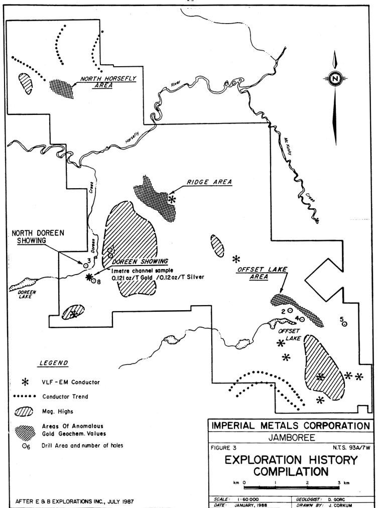
A program of soil and rock geochemical sampling and geological mapping was carried out. A total of 1760 soil samples were taken of which 103 returned gold values of greater than 25 ppb. The maximum value obtained was 5250 ppb Au. Over the course of geological mapping 230 rock chip samples were taken and geochemically analysed.
