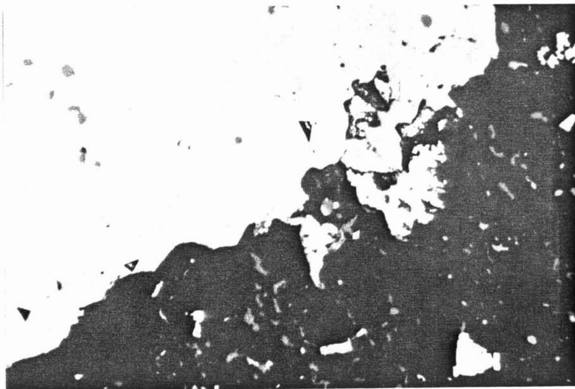
Plate 2: Sample RF4-1, Neg. 129-8. Tetrahedrite (Tetr) containing galena (Ga) and sphalerite (Sph) and native silver (Ag) (APPENDIX A).
