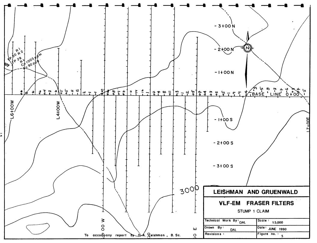
transmitter station, the unit is then held vertical. The coil now at right angles to the transmitting station is rotated to locate the field strength null position. The angle of rotation is then recorded either to the right (+) or left (-).
